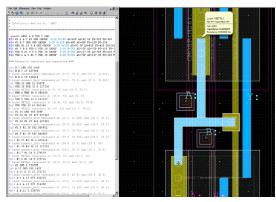
Hipex RC database provides visualization of parasitic elements on Expert layout view.
