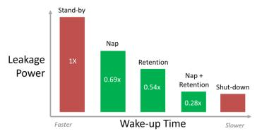
Leakage data for 4Kx32 instance@TT, 1.2V, 25°C
