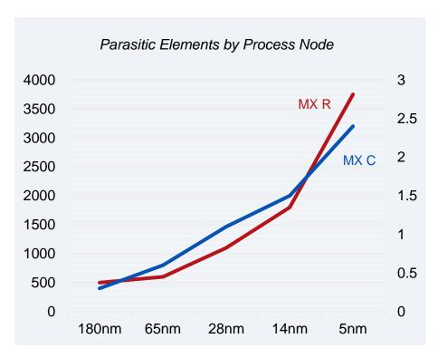
Number of parasitic resistors increased by 3.5X in between 28nm and 5nm.
