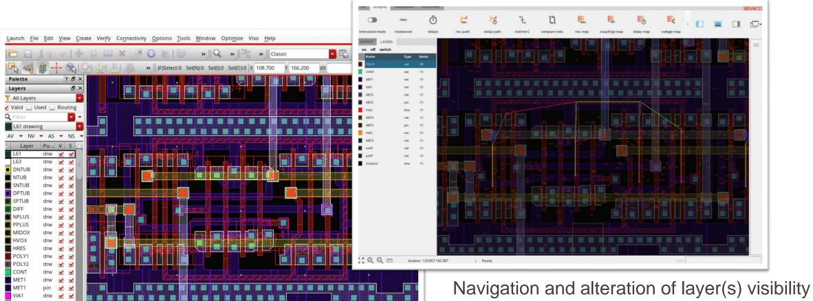
Navigation and alteration of layer(s) visibility in Viso is mirrored in Virtuoso, allowing a smooth exploration and optimization.
